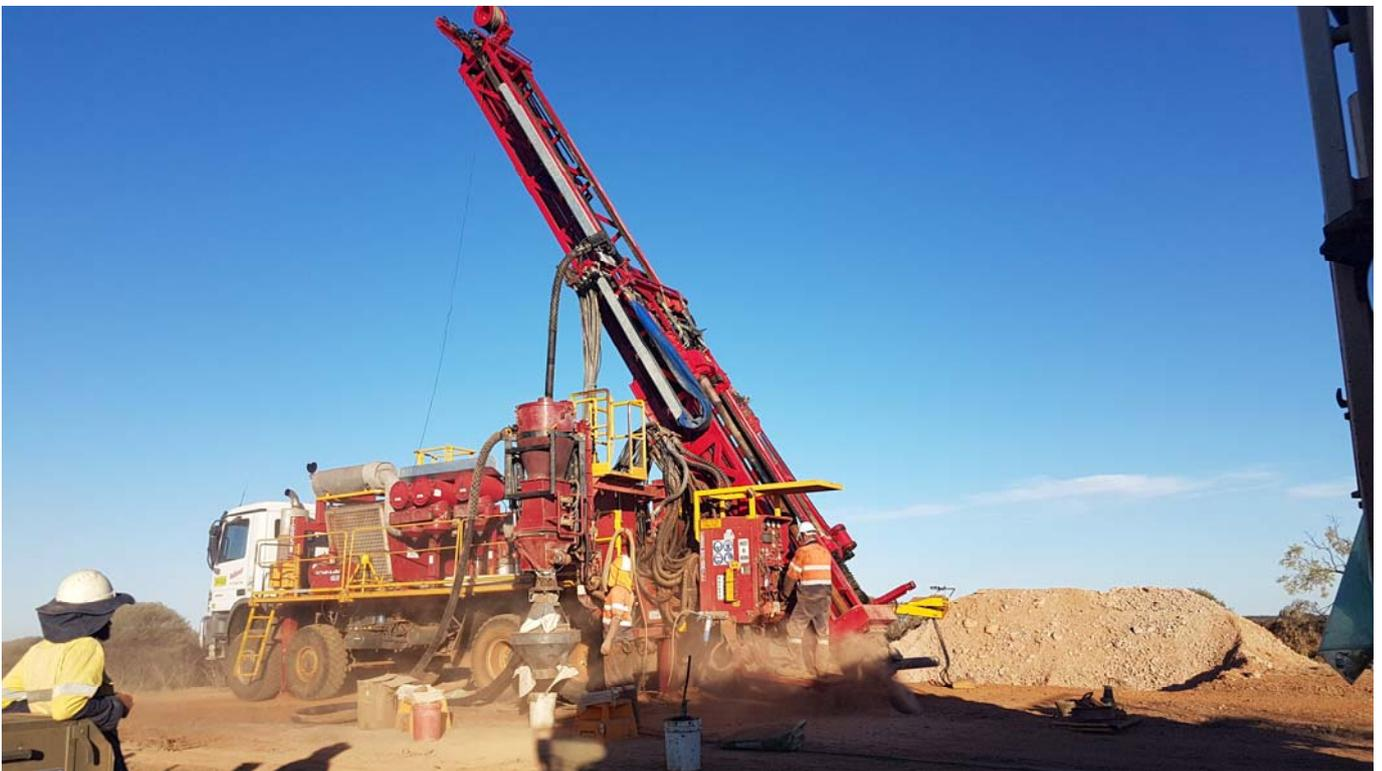
**Figure 3 – RC drilling underway at the Korong Prospect.**
