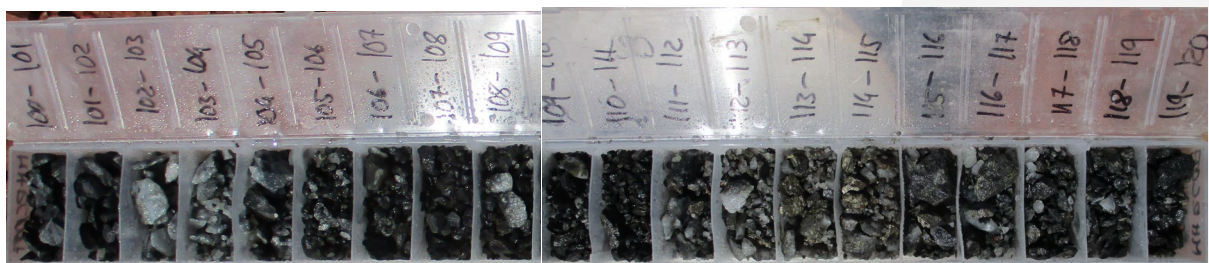
Photo 4. MHRC007 drill chips showing 46m of quartz copper sulphides from 71-117m.
